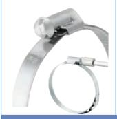
The NORMACLAMP® TORRO® Tamper-proof can only be mounted and dismounted by using a special tool. The specially designed screw head has three radial grooves, which means it cannot be adjusted with any commercially available tools. Automated assembly using a torque gun is particularly effective, as the special shape of the screw head allows for minimal misalignment or offset.
