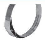
In this NORMACLAMP® TORRO® version, a spring insert is attached to the inside of the band. The spring insert is pretensioned during tightening, and the spring energy stored as a result of this ensures an automatic re-tensioning effect for an extended period. Even at extreme temperatures, this mechanism still enables a sufficient level of radial clamping force to be achieved.
